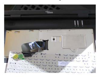
Lift RAM Cover and insert SIMM. A screw can be used to retain the cover.
