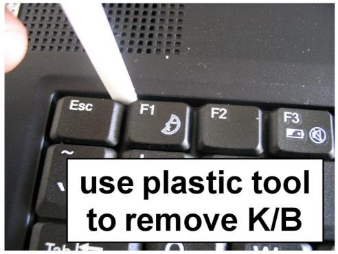
Release all 6 latches of the keyboard (please use something like the plastic tool to avoid damage and scratching)
